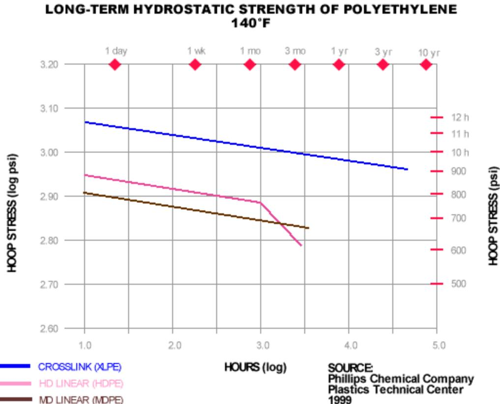
The rapid deterioration in properties is indicated by a “knee” in the curve of hoop strength versus time. Even high performance HDPE will develop a LTHS knee at around 1000 hours (log 3), and some MDPE products will have a knee in less than 10,000 hours (log 5). This type of performance substantially reduces the expected long-term performance at elevated temperatures. Crosslink has been tested to 50,000 hours at 140°F and shows no signs of a knee.
