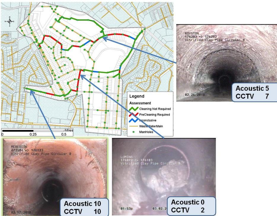
**Figure 3 GIS map for Basin 17-100, CMU Pilot Project location. Highlighted pipe segments represent locations evaluated with the SL-RAT acoustic inspection. The three CCTV snapshots illustrate comparison between the SL-RAT Blockage Assessment and the CCTV Blockage Assessment.**
