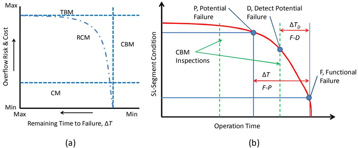
**Figure 6 (a) Regions of optimal application for four maintenance strategies (Lehtonen 2006); (b) Relationship between inspection and P-F in a CBM based maintenance strategy (Moubray 1997 and Wiseman et. al.).**
