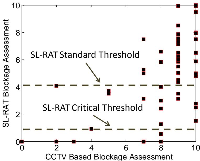
**Figure 4 Scatter plot comparing the CCTV Blockage Assessment with the SL-RAT Blockage Assessment for sewer line segments within the CMU Pilot Project. SL-RAT Thresholds used to discriminate between those pipe segments requiring additional maintenance (below the threshold) and those that do not (above the threshold).**
