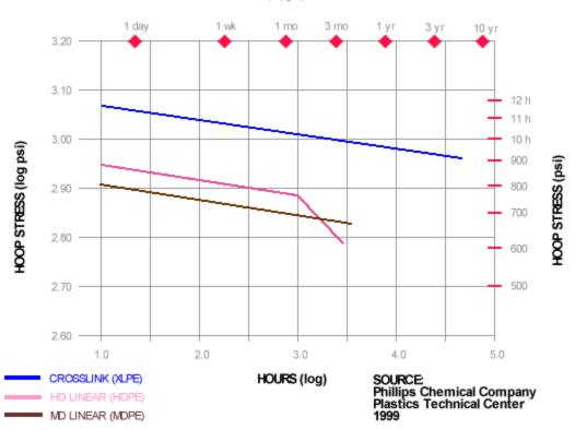
LONG-TERM HYDROSTATIC STRENGTH OF POLYETHYLENE 140°F
