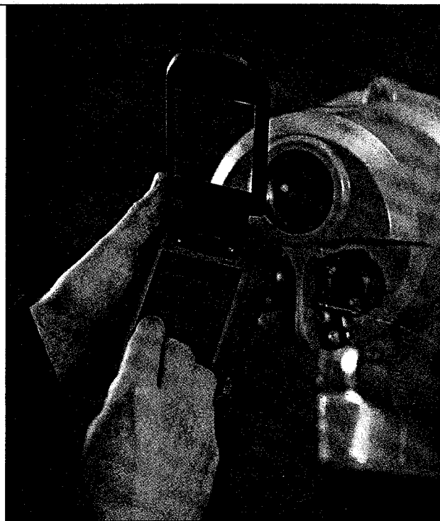
Figure 1. An actuator being set with a setting tool
