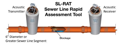
Figure 2 Concept and operation of the SL-RAT Acoustic Inspection System.
