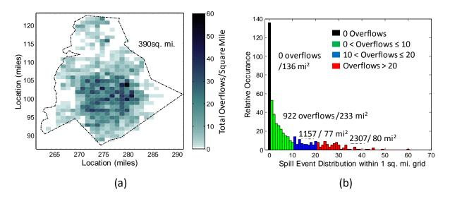
Figure 8 CMU SSO Evaluation for FY 00 through FY12 (a) Spatial representation of the overflows that occurred within one-mile-square grid over the thirteen year period; (b) Histogram of the number of overflows that occurred within a one-mile-square over the thirteen year period with the bar color distinguishing between three disjoint regions.
