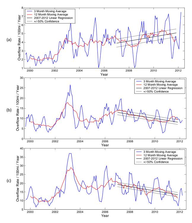
Figure 10 Both short time and long time moving averages of the Overflows / 100miles normalized to a one year time interval based on the CMU SSO data for FY 00 to FY 12 (a) Region I – 0<Overflows/SqMi $\leq$ 10; (b) Region II 10<Overflows/SqMi $\leq$ 20; (c) Region III Overflows/SqMi > 20.
