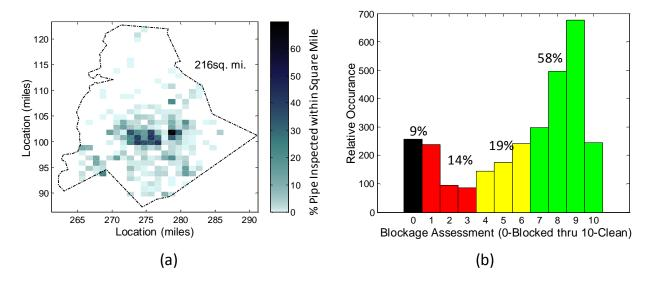
Figure 11 CMU Acoustic Inspection – (a) Spatial representation of the percentage of pipes inspected within each square mile grid; (b) Histogram of the blockage assessment.
